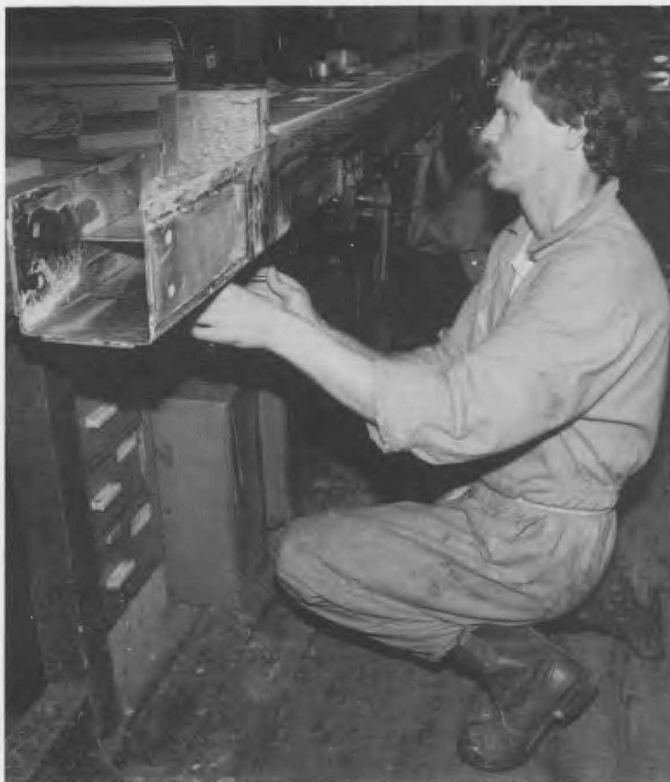
Fig. 3. The U-shaped core barrel is placed horizontally in two carpenter's vices which are attached to a work bench. The upper side of the barrel which serves as the lid has been removed. The sediment surface is protected by a square plate which prevents it from slumping. By turning the threaded T-bars on the underside of the barrel, the double bottom is forced upwards and extrudes the sediment. In this photograph, half of the core has been removed and a series of plastic trays has been pressed into the core. Clearly visible are the reinforcement plates where the barrel is connected to the core head.
