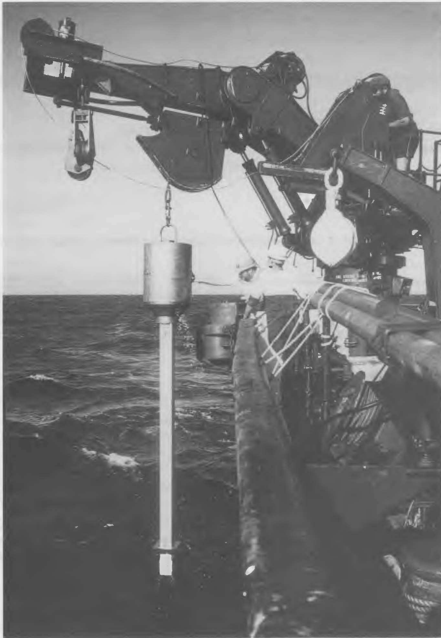
Fig. 1. The full 3 m long kasten core returning from the seabed. At the top of the corer is a 750 kg weight which is connected to the barrel by the core head. At the bottom of the barrel is the sliding weight and the core catcher.
